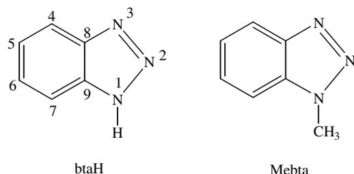
Fig. 1. Benzotriazole (btaH) and 1-methylbenzotriazole (Mebta).
