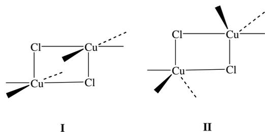
Scheme 1. The two common structural types of the bis( $\mu$ -chloro) copper(II) dimers: square-pyramidal apical-basal dimers (**I**) and trigonal-bipyramidal axial-equatorial dimers (**II**).
