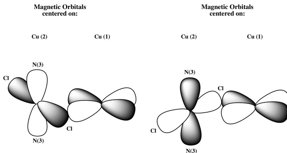
Scheme 3. Accidental orthogonality of the sequential magnetic orbitals in **3**, accounting for its intrachain ferromagnetic exchange interaction.
